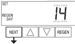
**Step 3I** – Day Override: When volume capacity is set to “oFF”, sets the number of days between regenerations. When volume capacity is set to AUTO or to a volume, sets the maximum number of days between regenerations. If value set to “oFF”, regeneration initiation is triggered solely by volume used. If value is set in days (allowable range from 1 to 28) regeneration initiation will be called for on that day regardless of actual water usage. Set Day Override using ▲ or ▼:
