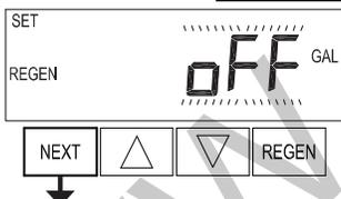
**Step 5F** - Set Regeneration trigger using ▲ or ▼. If value is set to:
