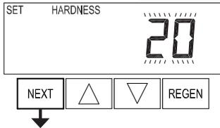
**Step 2I** – Hardness: Set the amount of influent hardness using ▲ or ▼. This display will not be viewed if FILTERING BACKWASH or FILTERING REGEN is selected in Step 2F or if “oFF” or a number was selected in Step 1IS.
