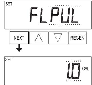
**Step 4CS** – Selecting the use of an outside signal to initiate a regeneration: Selection only matters if a connection is made to the two pin connector labeled DP SWITCH located on the printed circuit board. Following is an explanation of the options:
