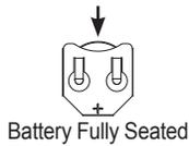
Correct Battery Orientation → ← Battery replacement is 3 volt lithium coin cell type 2032.
