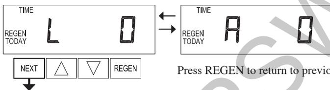
**Step 12D** – MAV Drive History in the direction of retracted piston rod position. Display will only be shown if 1.0Γ is selected in Step 2CS, or OFF is not selected in Step 5CS. Up to a four digit number will appear after the “L” which stands for latest and “A” which stands for average. Drive time is measured in 1/100 of a second; i.e., a 17.10 second move is displayed as “1710”. Press NEXT at any time to go to Step 13D. Press REGEN to return to previous step.
