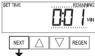
**Step 15S** – Set Relay Deactivate Time using ▲ or ▼.
