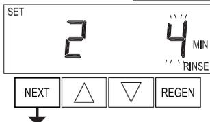
**Step 4F** - Select the time for the second cycle using ▲ or ▼. If Step 2F is set to FILTERING REGEN, press NEXT to program the rest of the cycle times. If Step 2F is set to FILTERING BACKWASH, press NEXT to go to Step 5F. Press REGEN to return to previous step.
