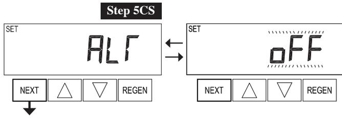
**Step 5CS** – This display will not appear if 1.0Γ was selected in Step 2CS. Allows selection of one of the following using ▲ or ▼:
