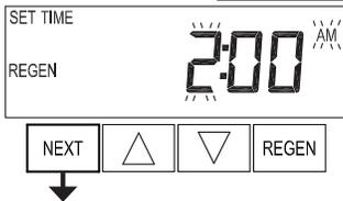
**Step 4I** – Next Regeneration Time (hour): Set the hour of day for regeneration using ▲ or ▼. The default time is 2:00. This display will show “REGEN on 0 GAL” if “on 0” is selected in Set Regeneration Time Option in OEM Softener System Setup or OEM Filter System Setup.
