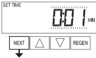
**Step 14S** – Set Relay Actuation Time or Gallons using ▲ or ▼. The choices are:
