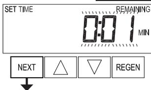
**Step 9F** – Set Relay Deactivate Time using ▲ or ▼.
