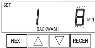
**Step 3F** - Select the time for the first cycle using ▲ or ▼. Press NEXT to go to Step 4F. Press REGEN to return to previous step.
