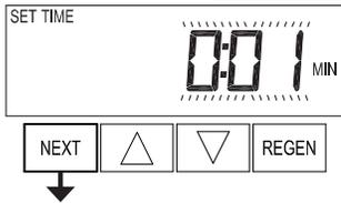
**Step 8F** – Set Relay Actuation Time or Gallons using ▲ or ▼. The choices are:
