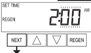
**Step 5I** – Next Regeneration Time (minutes): Set the minutes of day for regeneration using ▲ or ▼. This display will not be shown if “on 0” is selected in Set Regeneration Time Option in OEM Softener System Setup or OEM Filter System Setup.
